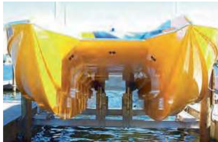
TUNNEL HULL BRACKETS
